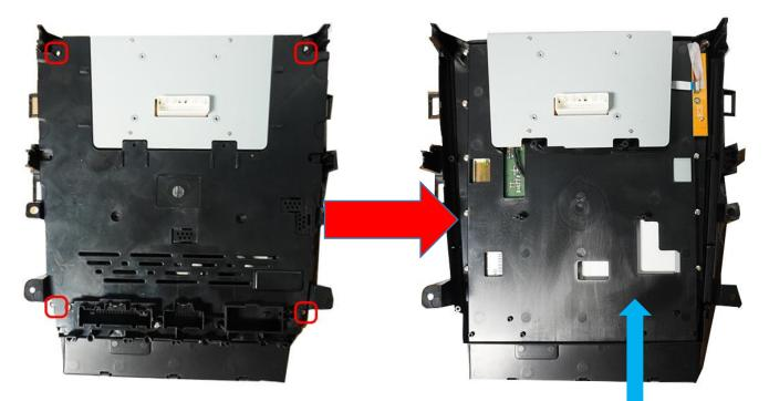
2. Unmount AC board from Original Display and place it on Android Display
