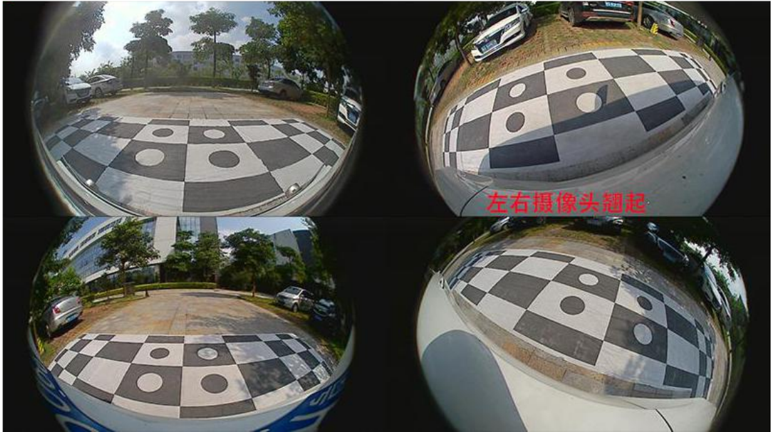
The Angle of the left camera and right camera is not right, so the cloth in the picture is crooked
