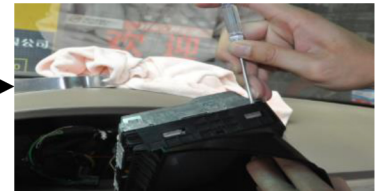
12. Pried loose the Plastic cover with a flat screwdriver
