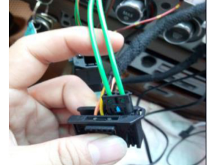
20. Connect the Optic Fiber cable into our adapter.
