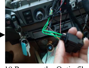
19. Remove the Optic fiber cable from screen socket and Connect the socket with our adapter
