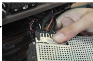
22. Insert Android Power harness into original Host.
