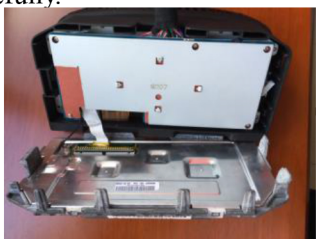
17. Connect the socket from Android device with aluminum back cover
