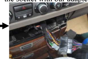
23. Connect the original power harness with Android Power harness.
