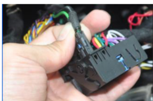
21. Take out the Optic fiber cable and plug it into the factory harness.
