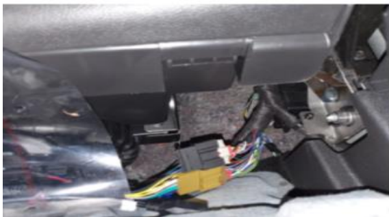
POWER PLUGS IN HAND GLOVE COMPARTMENT CONNECT TO PLUGS 1 & 2
