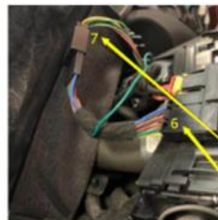
POWER PLUGS IN HAND GLOVE COMPARTMENT CONNECT TO PLUGS 6 & 7
